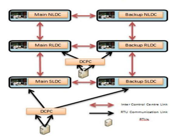
The Backup SLDC shall be a fully functional replica of the Main SLDC (with minor changes) so that it can function as a full fledged SLDC in case of any disaster. During normal course, it shall share the duties of main SLDC also.
